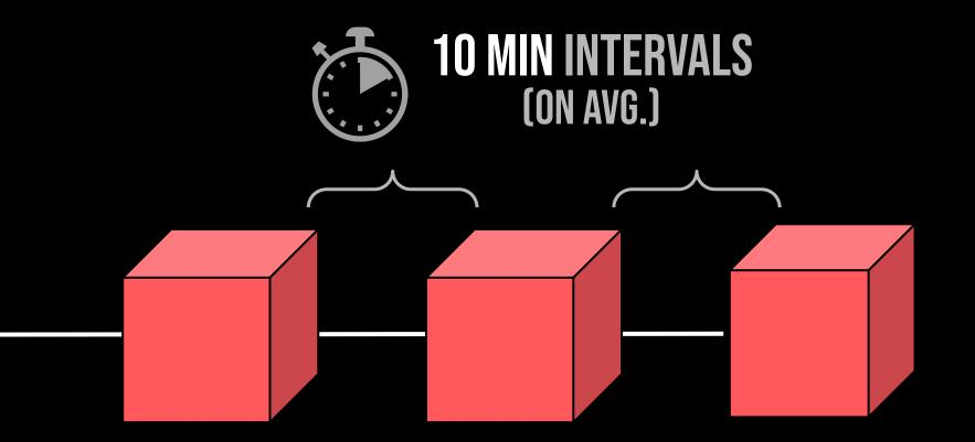
Block production is programmed to occur at a regular interval. If block times stray too far from the targeted 10 minute interval, the level of difficulty adjusts upwards or downwards.
